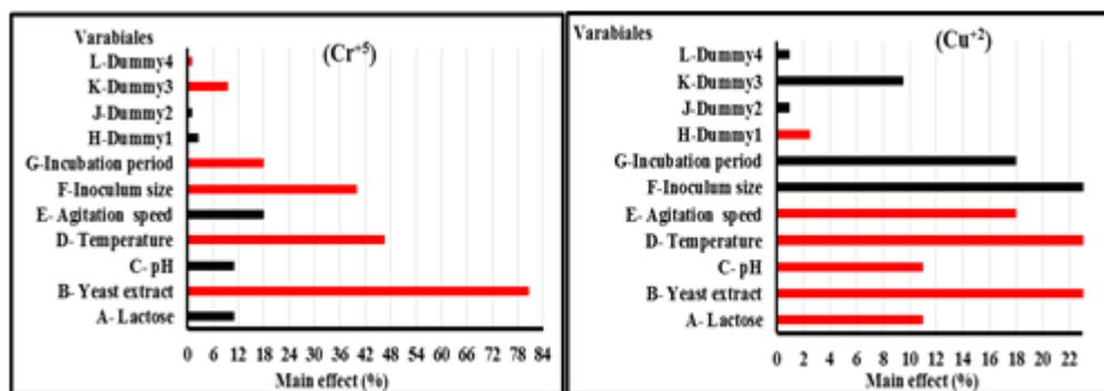
**Figure 5.** Pareto graph showing contribution effect % of different variables on heavy metals removal by *A. terreus* FR1 based on the observation of Plackett-Burman design (the black color represents positive effects and the red color represents negative effects).
