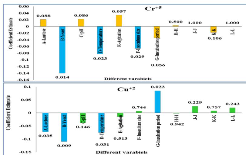
**Figure 4.** The extent of positive and negative effects of the eleven factors on heavy metals removal by *A. terreus* FR1 and the corresponding p-values (number above each bar) of the factors showing their significance (if  $p < 0.05$ ) based on ANOVA according to the Plackett-Burman experimental results. The blue bars indicate the positively significant factors.
