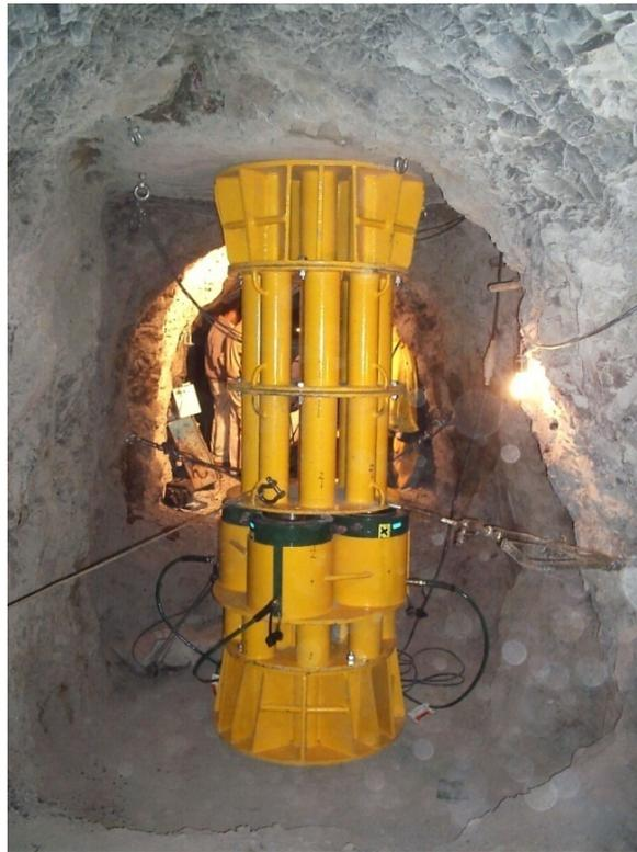
**Figure 2.** Plate jacking test operation.
